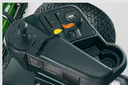
CommandARM control panel Combination of armrest and control centre keeps all vital functions (like lights, lift/lower lever, PTO, throttle and optional cruise control) within easy reach.
