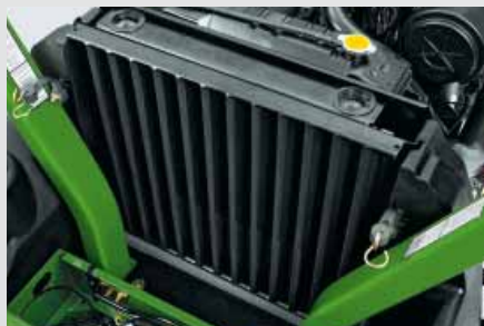
Daily service, simplified All checks are located on the left hand side and the oil cooler tilts out for easy cleaning.
